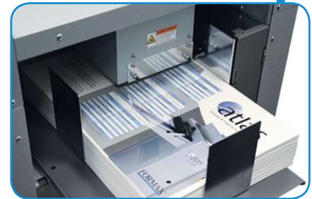
Upper-belt tri-suction feed system for accurate feeding of large & heavy stocks
